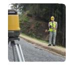
Easy guidance User-friendly prism re-acquisition with color coded guide light.
